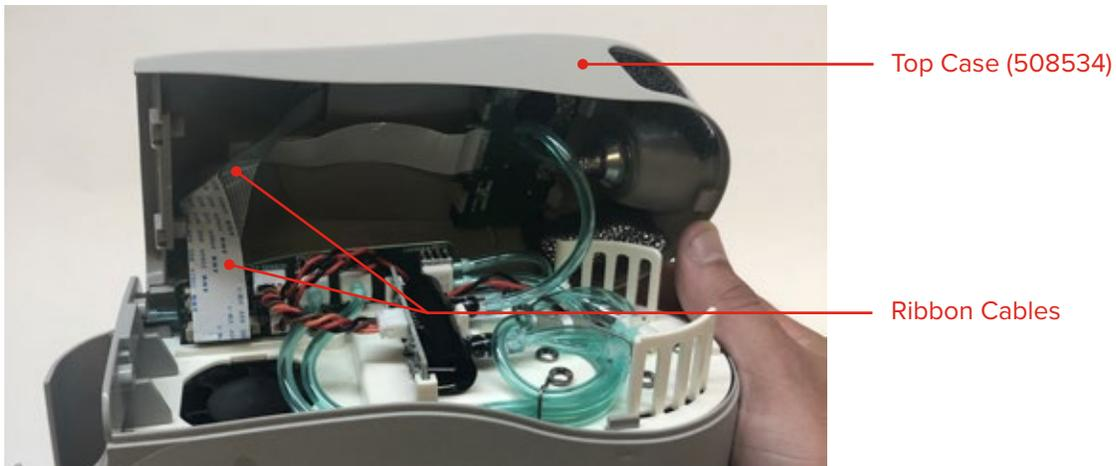
3. Disconnect the wires from the PC board to the O2 sensor (508419).
