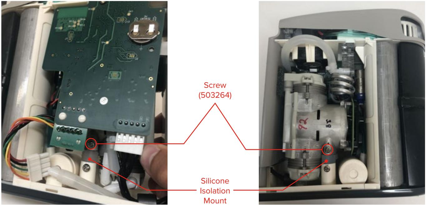
8. Remove the compressor assembly (508525) from the silicone isolation mount (508554).
