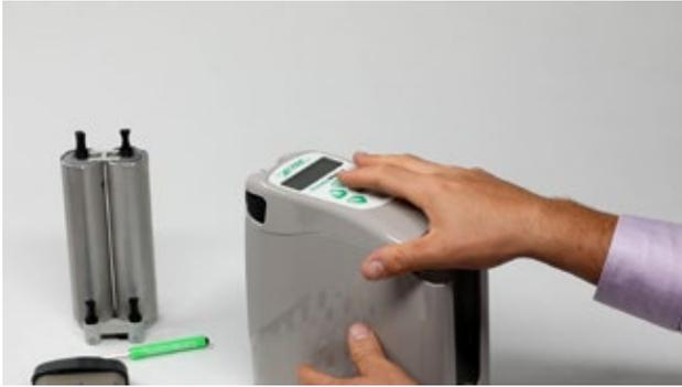
2. Turn unit upside down, and place on soft surface. Remove screws and bottom cover.
