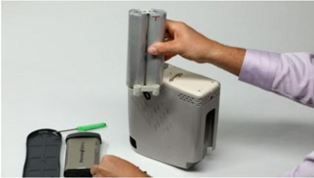
2. Gently push until sieve bed replacement is fully seated, flush with bottom surface. Replace bottom cover and secure screws.
