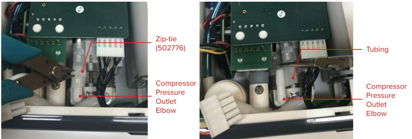
6. Disconnect the tubing from the compressor pressure inlet elbow (505806).
