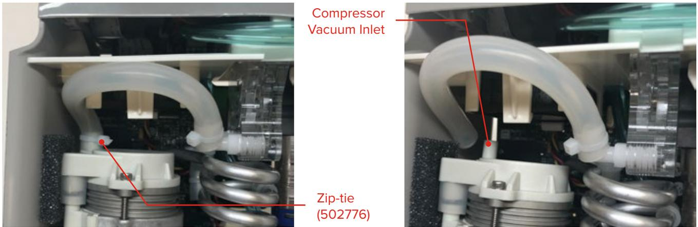
5. Cut and remove the zip-tie (502776) from the compressor pressure outlet elbow (505806). Disconnect the tubing from the compressor pressure outlet elbow (505806).
