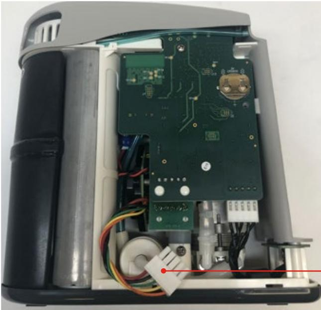
Compressor Assembly Wires
