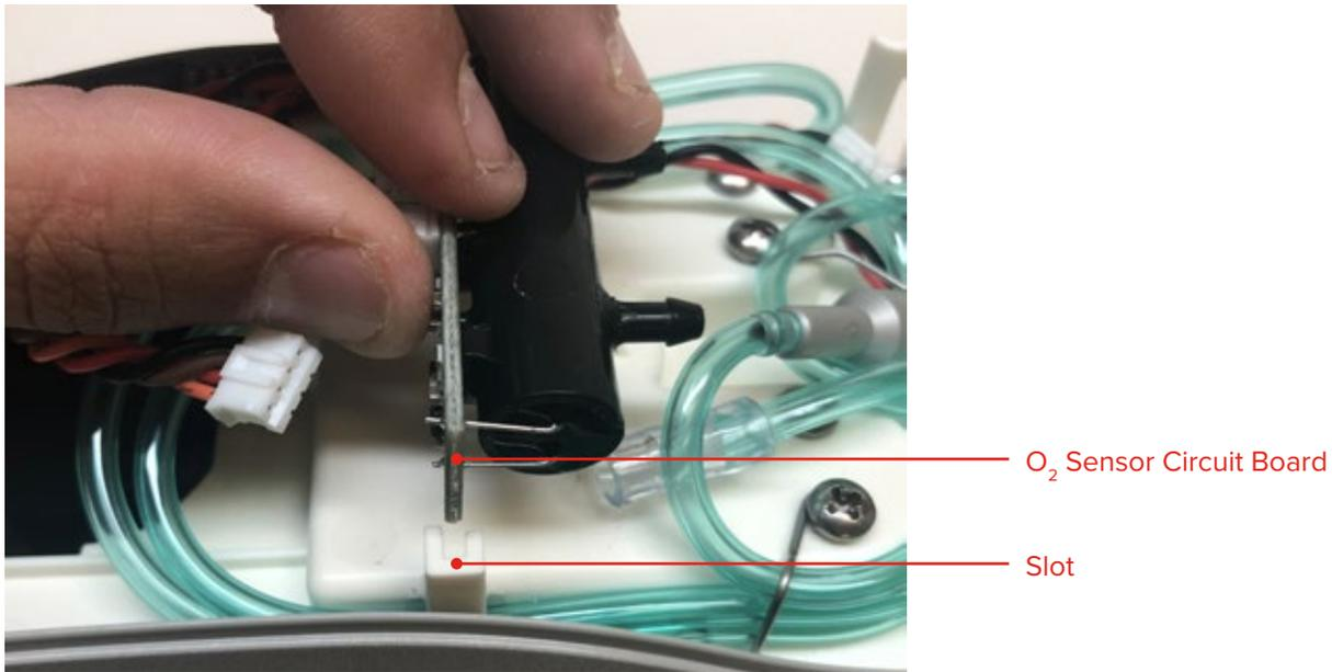
2. Slide the O<sub>2</sub> sensor into the slots and press until the O<sub>2</sub> sensor locks into place with the locking tab.
