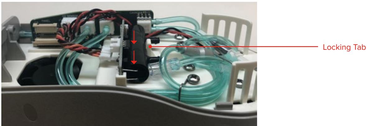
3. Connect the wires from the PC board to the O<sub>2</sub> sensor.
