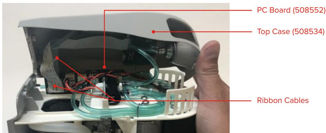
6. On the PC Board (508552), disconnect the wires that go to the O2 Sensor (508419), dose valve (518166), and crossover valve (508568).
