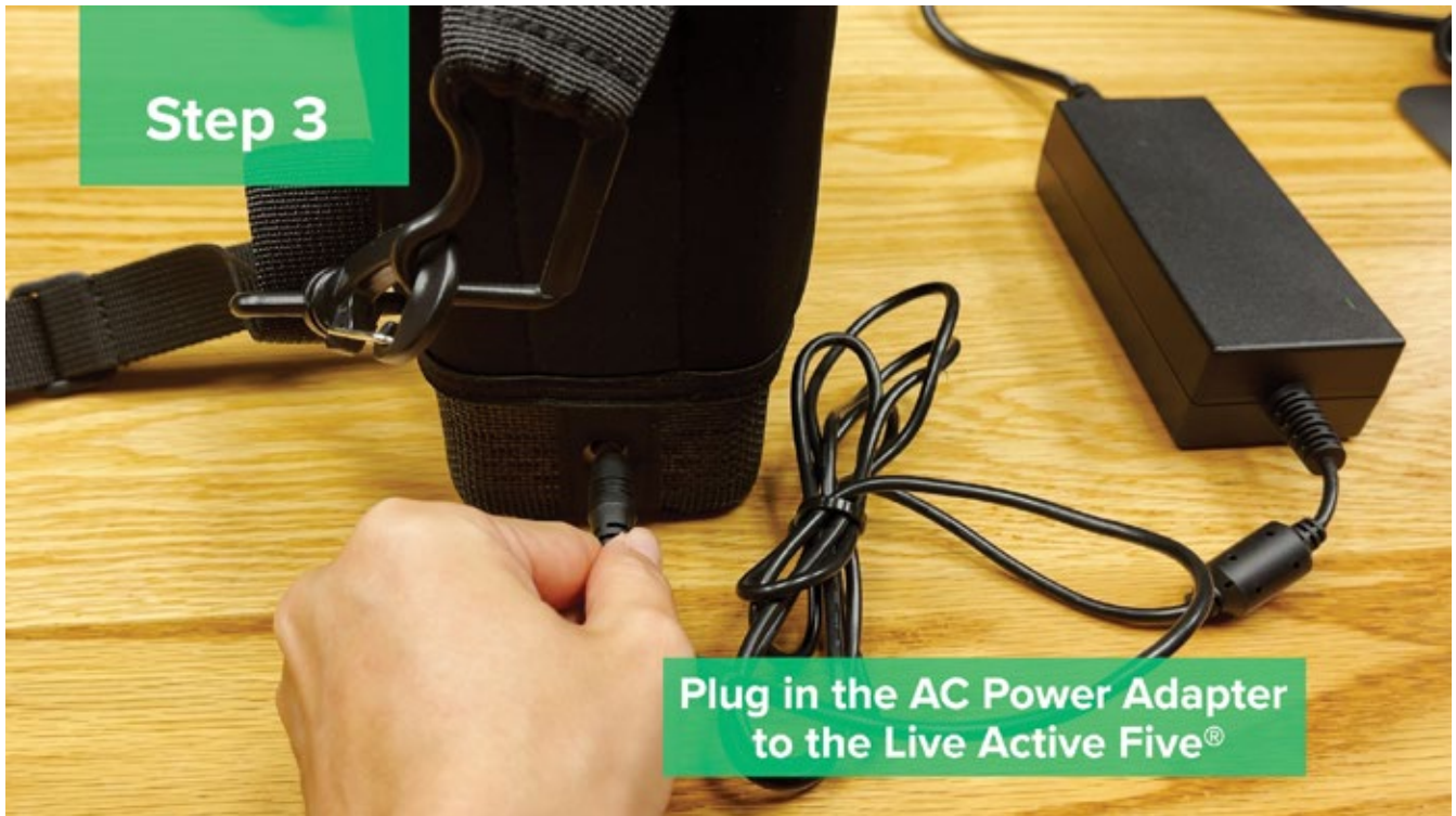
Step 3: Plug in the AC Power Adapter to the portable oxygen concentrator.
